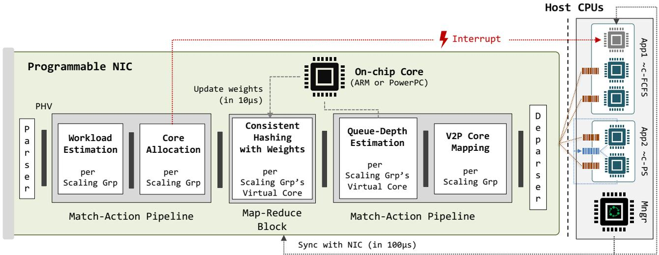
Figure 2: eRSS’s NIC pipeline performs core and packet scheduling for each incoming packet. The on-chip core updates weights at approximately  $10\ \mu\text{s}$  intervals, and the software manager syncs runtime state (e.g., the true queue depths and per-scaling group core mapping) with the NIC at  $100\ \mu\text{s}$  intervals.
