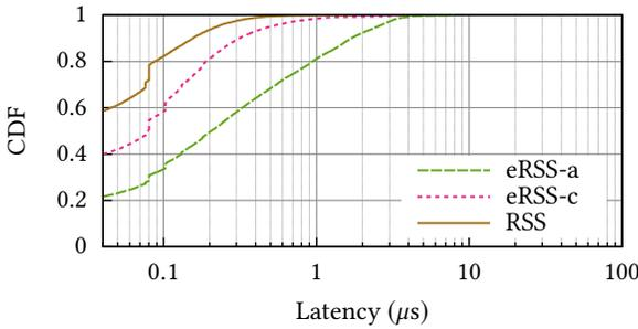
Figure 4: eRSS’s 99th-percentile (tail) latencies, modeled as a function of queuing delay.
