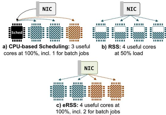
**Figure 1: eRSS achieves better core utilization than RSS-only techniques without dedicating a CPU core for packet forwarding.**
